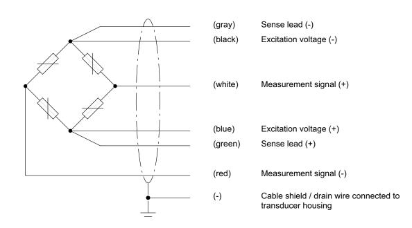
With this cable assignment, the output voltage at the measuring amplifier is positive in the tensile direction when the transducer is loaded.
