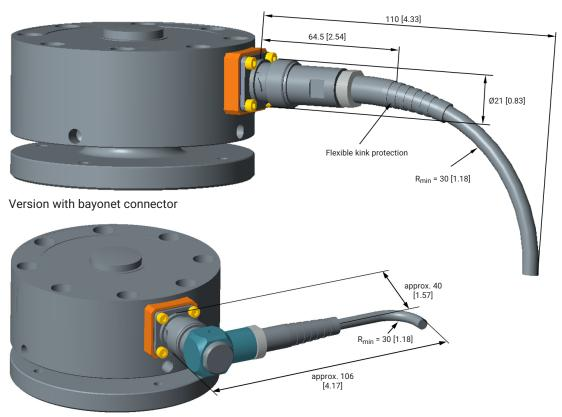
Version with angular plug Dimensions in mm [inch]
