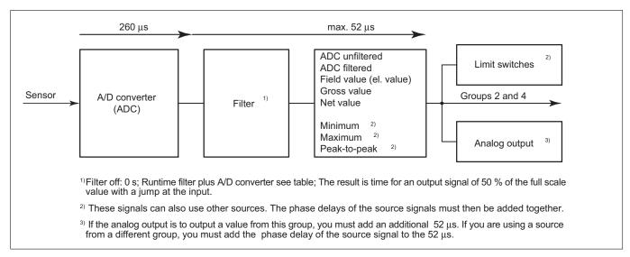
Fig. 1: Minimum phase delays for group 1: 52 ms plus A/D converter conversion time plus filter runtime
