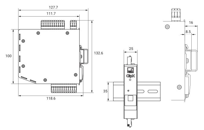
**Note**: ClipX devices can be manually fitted to the DIN rail and removed without the need for tools. To help with construction, ready-prepared ePLAN macros (no license required) and 3D STEP files are available free of charge at https://www.hbm.com/ClipX.
