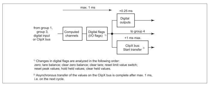
Fig. 2: Maximum phase delay for group 2: 1 ms
