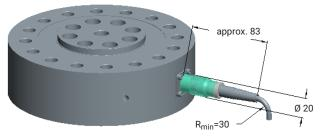
Connection cable KAB-158 with screw connector, compatible with a MIL-C-26482 series 1 connector
